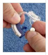
their size, it's a good idea to change and replace batteries above a table or desk to reduce the risk of dropping the instrument or battery.
