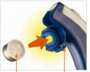
Place the new battery in the compartment with the plus (+) sign facing up.
