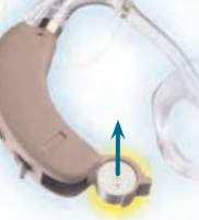
Remove the existing battery by pushing it out the top of the door.
