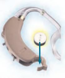
Close the battery compartment by swinging the door until it snaps securely. NEVER FORCE THE DOOR SHUT. This could result in serious damage. If the door will not close securely, check that the battery is placed properly in the compartment.
