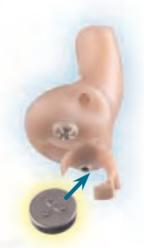
Close the battery compartment by swinging the door until it snaps securely. NEVER FORCE THE DOOR SHUT This could result in serious damage. If the door will not close securely, check that the battery is placed properly in the compartment.
