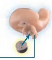
Close the battery compartment by swinging the door until it snaps securely. NEVER FORCE THE DOOR SHUT. This could result in serious damage. If the door will not close securely, check that the battery is placed properly in the compartment.
