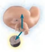
Remove the existing battery either by pushing it out the top of the door, or pulling it straight out.
