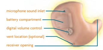
Your Libra CE Digital In-The-Ear (ITE) has been custom-made with the precise electronic circuitry controls to match your particular hearing requirements.
